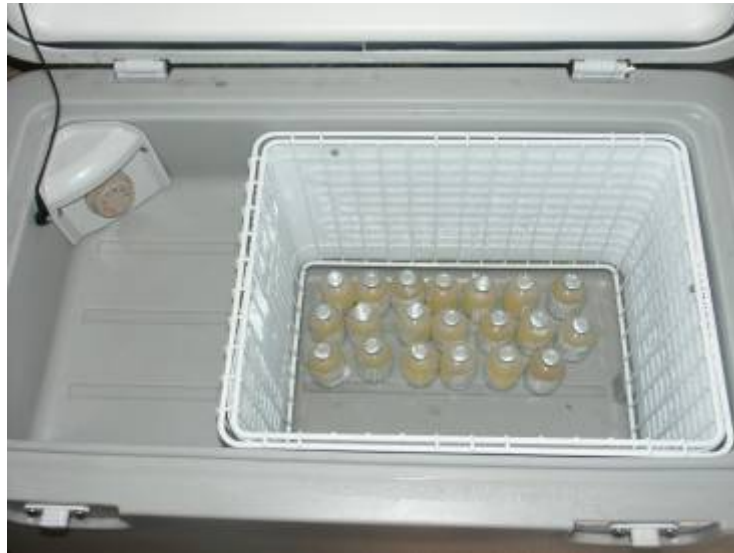
Solar PV powered Vaccine storage (Courtesy by Sunlabob Co.)
