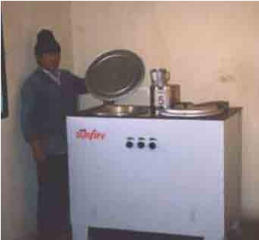
Figure 8: flat plate collector cooker (GTZ publication, 2007)
